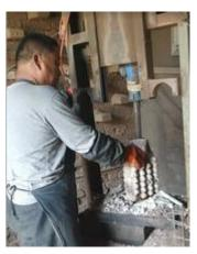
When the metal has cooled and solidified, the ceramic shell will be broken off by vibration or knock-out machine.
