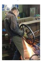
After the casting was cut off. The casting pouring part will be grind ed carefully.
