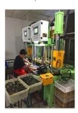
The wax is be injected by machine. Wax design of the desired castings are produced by injection molding. These process is called patterns.
